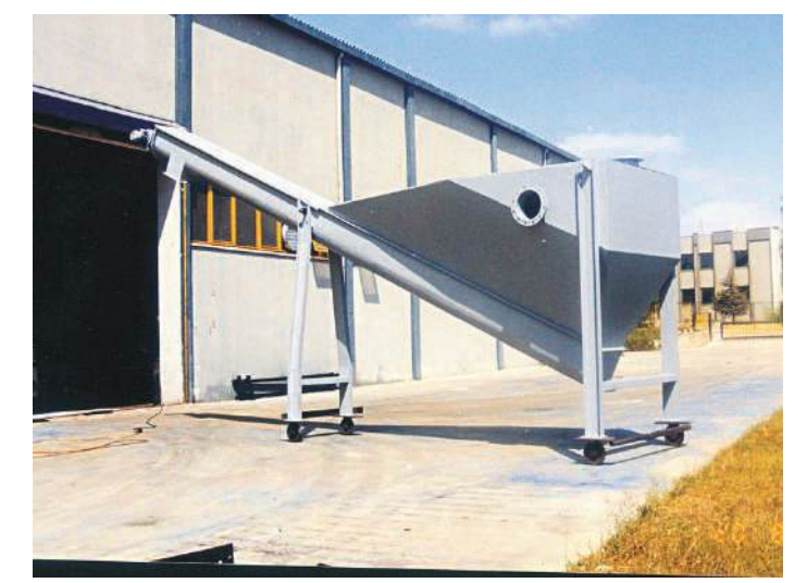
Grit Removal System
