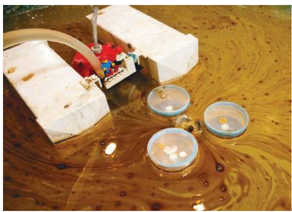
Oil Skimmer (Fog & Scum Removal)
