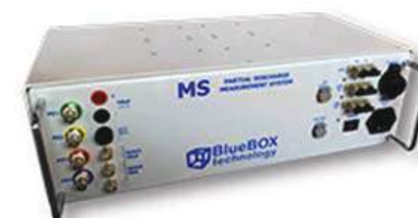
Cable Partial Discharge Monitoring System
