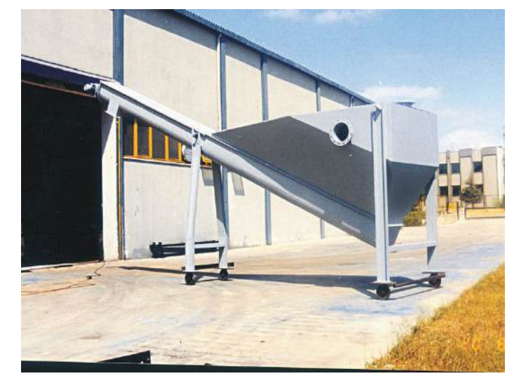
Grit Removal System
